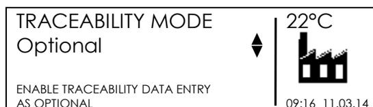
Select by (▲)(▼) the traceability mode and press START/OK (I) to confirm the setting. To cancel the operation press STOP/ESC (O).
