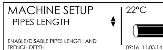
Select by (▲)(▼) buttons if You want to enable or disable the functionality and push START/OK (I) to confirm the setting.
