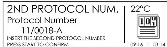
The second fusion number consist of four numerical positions and one position separated by a minus sign.
