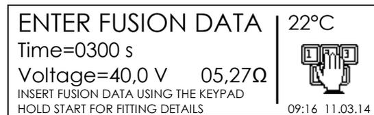
In this case, the user has to press the MENU button when the fitting is connected and the machine is waiting for the barcode entry. Set by (▲)(▼) the fusion time value, move the cursor to the next digits by (◀)(▶) and set the other values, push START/OK (I) to confirm the content and move to the next field. Then set by (▲)(▼) the fusion voltage value. Press START/OK (I) to confirm the setting and move forward to the fusion process.
