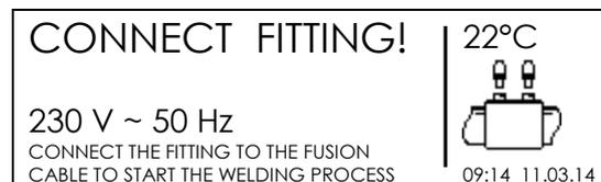
Meanwhile, the display shows the information about ambient temperature, current date/time, voltage and frequency values of the power supply applied to the electro-fusion unit, when GPS coordinates will be available a satellite icon in the top right corner.
