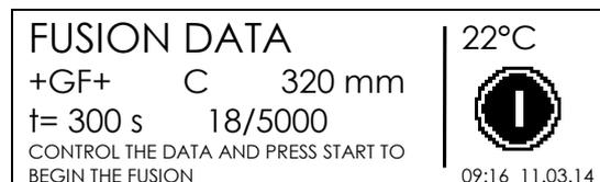
If the value of the fitting resistance doesn't match with the barcode data, the display shows an error message. Then the user has press the STOP/ESC (O) button, and re-enter the data.
