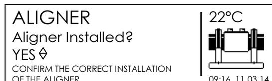
If ALIGNER CHECK alert is activated, the display shows a message which requires to declare if the aligner is properly used and installed. By pressing the UP/DOWN buttons the user can switch between YES/NO, as soon as the selection has done, press the START/OK (I) to proceed.
