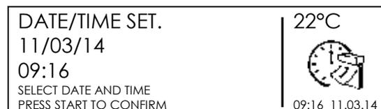
Select by (▲)(▼) the desired value; move the cursor position by (◀)(▶) to continue the insertion. When insertion is completed, press START/OK ( I ) to confirm the setting. To cancel instead the operation press STOP/ESC (O).
