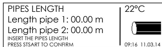
In both cases, the operator may insert manually the digits, just pushing the (▶) button to enter in edit mode, and then using the (▲)(▼) buttons to select the digits and the (◀)(▶) to move through the different fields. At the end the START/OK (I) button is used to confirm the content.
