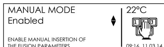
If the manual mode will be enabled, the user can insert manually the fusion data pressing the MENU button as soon as the machine detect the fitting resistance.
